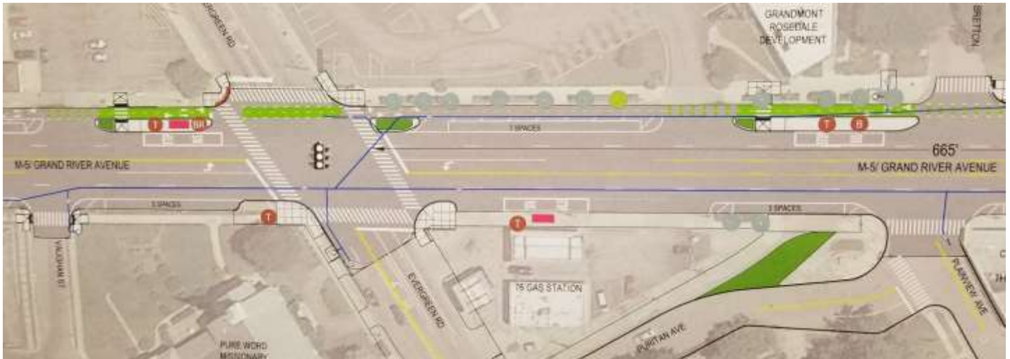
Grand River east of Evergreen. Note the bus island at Brettton on the north side. Buses will stop in the traffic lane at islands. The two-way bike lane is between the parking lane and the curb. Puritan and Plainview has been redesigned. Right turn lanes have been eliminated. The red rectangles indicate solar-powered bus shelters.
